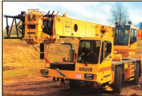
35 ton crane travelling through steep terrain
